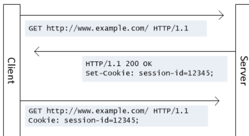
Figure 14. HTTP cookie tracking mechanism between a client (web browser) and a server.
